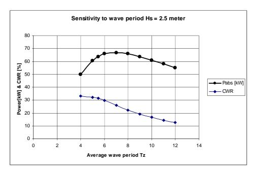
Fig 6. Power production in a sea state with significant wave height Hs = 2,5 meter at different average wave periods Tz and variation of Capture with ratio in irregular sea.
