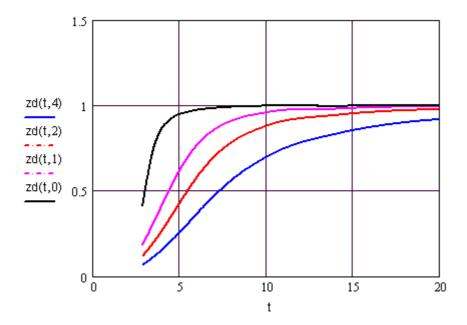
Figure 11. Float response as function of wave period for different values of external damping.
