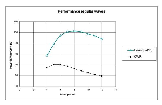
Figure 4. Power production in regular waves of height 2 meter and capture with ratio.
