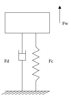
Fig 10. Principle of oscillating float system
