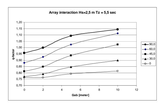
Figure 8. Plot of the results of the array calculations showing the q-factor as a function of the gab between the floats for different angles of incidence.
