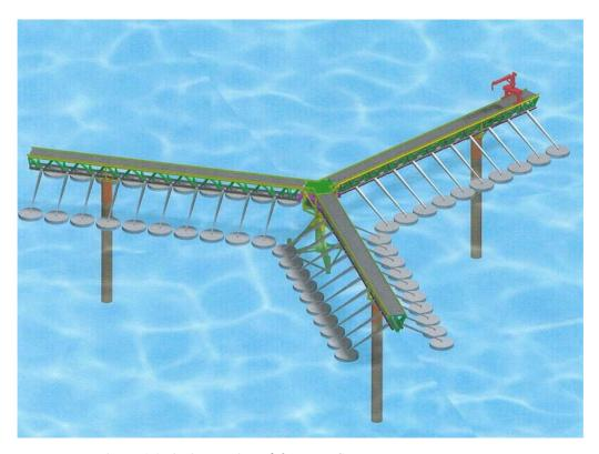
Figure 1 Artist impression of the Wave Star wave energy converter.
