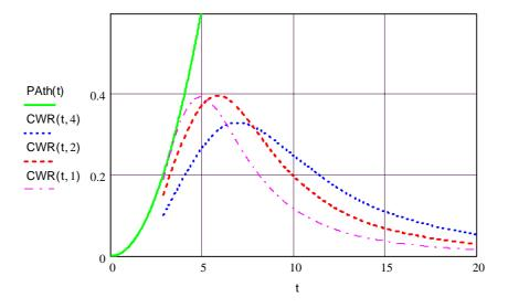
Figure 12. Capture width ratios CWR as function of wave period for different values of the external damping. The green curve shows the theoretical capture width ratio for Point Absorbers.
