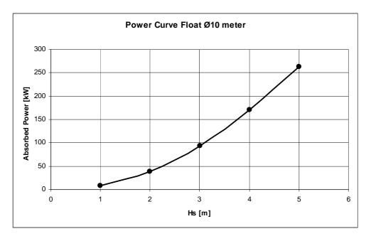
Figure 5. Theoretical power curve for a single 10-meter diameter float
