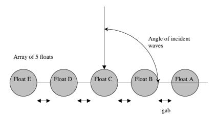
Figure 7. Definition of incident wave direction – (If the angle of incidence is 90 degree then the floats in long crested waves will move identically up and down.)
